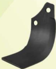
GYROVATOR TYPE (70 x 7/8 mm) Center 44 mm Thickness : 7 / 8 mm Hole : 14.5 / 12.5 mm
