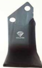
L-TYPE (80x7 mm) Center 46 mm / 57 mm Thickness : 7 / 8 / 9 mm Hole : 14.5 / 12.5 / 11.5mm
